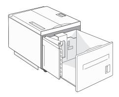
2 If loading print media with a different width or length, adjust the width and length guides.
